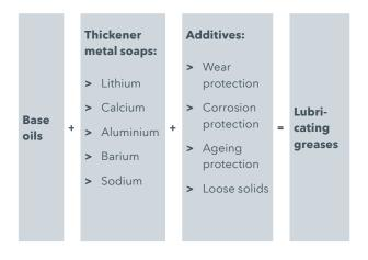
The use of different additives causes great changes in lubricant characteristics. This explains the large number of lubricants available: The WIRTGEN GROUP offers you greases optimally matched to your machine.
