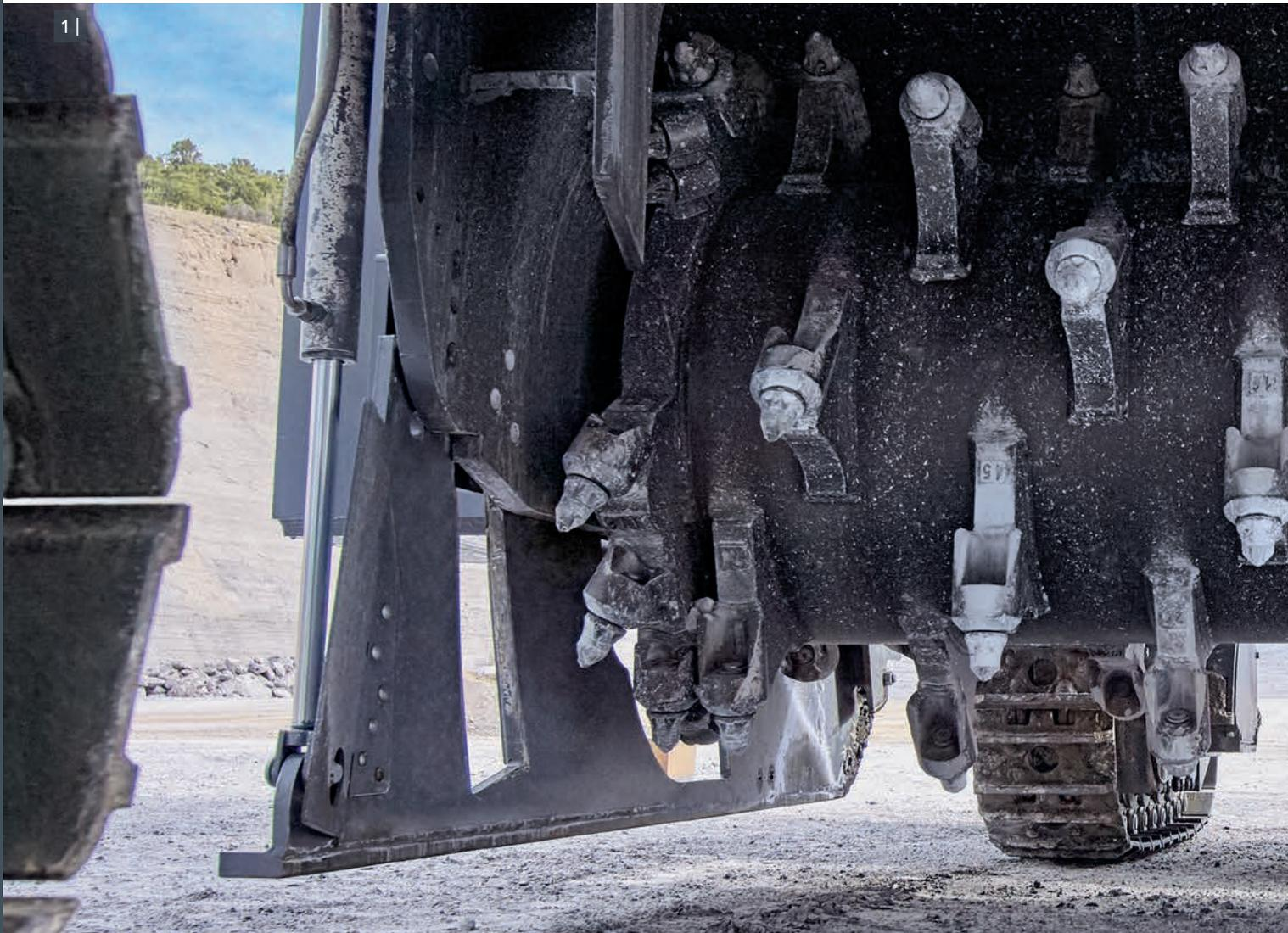
1 | The picks are arranged in a specific pattern tailored to the windrowing method.
