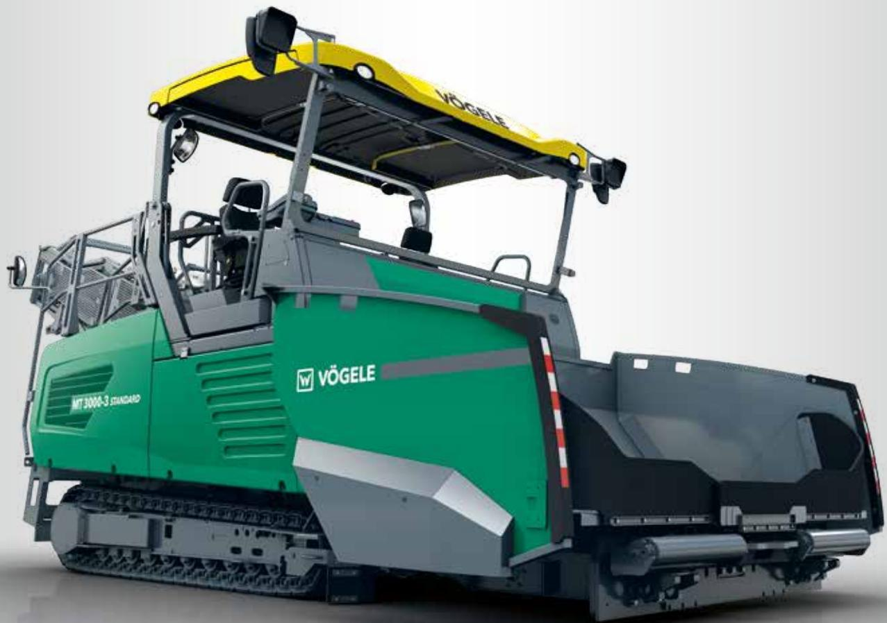
Maximum conveying capacity 1,200 t/h
